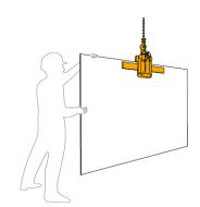
\* The additional width of this clamp will prevent the slab from bending during handling to, thus, prevent undesirable breakage. This clamp is available through Lotte & our distributor partners. Contact Lotte for more details.
