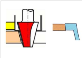
③ Rout the cutout to a 15 degree bevel with an oblique router bit
