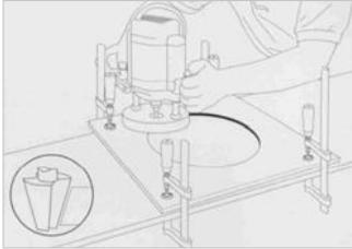
① Clamp the bowls template into position on the top of the sheet
