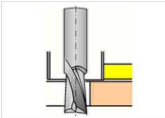
② Rout the bowls cutout with a 30mm template guide and use the router in one motion
